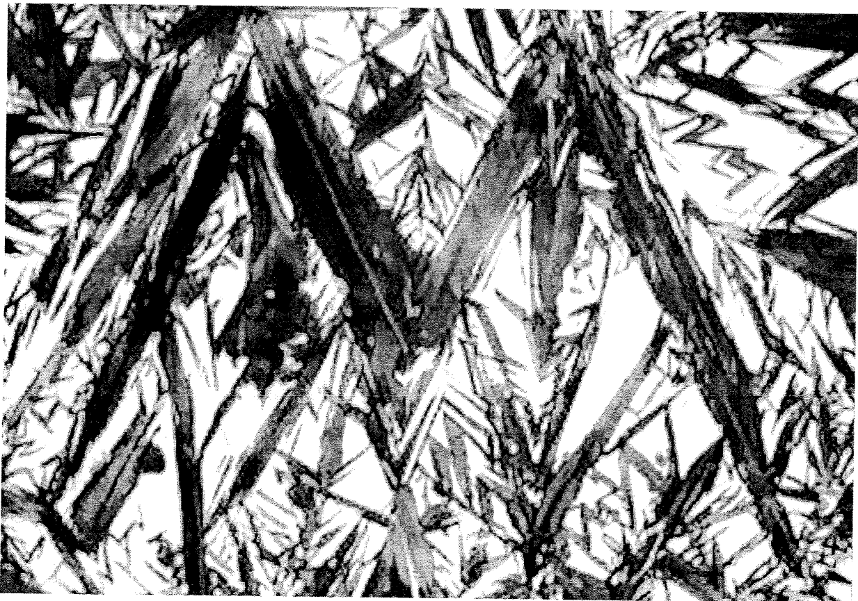
Fig. 1.3. Optical micrograph of spear-like \gamma' martensite in Cu-14.2 mass% Al-4.2 mass% Ni alloy.
