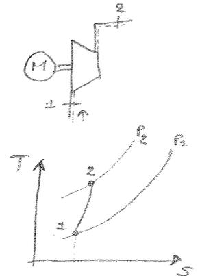
$$\dot{Q} + \dot{L}_i = \Delta h + \underbrace{\Delta E_c}_{\approx 0} = \underbrace{\Delta h^{\circ}}_{\Delta h_{\text{mecc}}} \approx \Delta h$$
