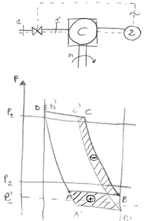
$$Q_c = \frac{m^*}{m^* - 1} P_B V_B \left( \beta_i^{\frac{m^* - 1}{m^*}} - 1 \right) - \frac{m^*}{m^* - 1} P_A V_A \left( \beta_i^{\frac{m^* - 1}{m^*}} - 1 \right)$$
