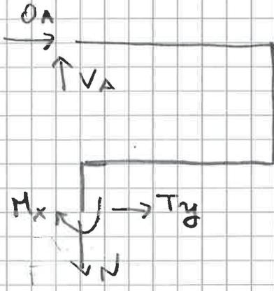
$$\begin{aligned} O_A + T_y &= 0 \\ V_A - N &= 0 & N &= V_A = -F \\ M_x + O_A \left( z - \frac{3}{2}e \right) &= 0 \end{aligned}$$
