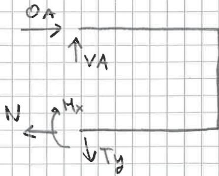
$$\begin{aligned} \uparrow \quad V_A - T_y &= 0 & T_y &= V_A = -F \\ \rightarrow \quad O_A - N &= 0 & N &= 0 \\ \curvearrowright \quad M_x + V_A z &= 0 & M_x &= Fz \end{aligned}$$
