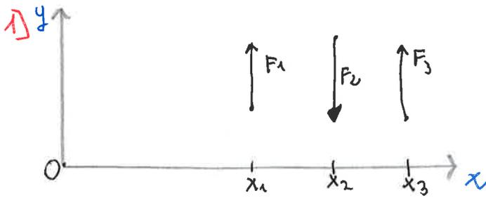
$$\begin{aligned} F_1 &= 500 \text{ N} \\ F_2 &= 800 \text{ N} \\ F_3 &= 1000 \text{ N} \\ x_1 &= 5 \text{ m} \\ x_2 &= 7 \text{ m} \\ x_3 &= 8 \text{ m} \end{aligned}$$
