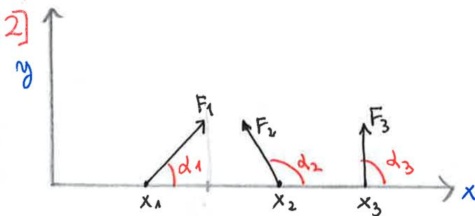
$$\begin{aligned} F_1 &= 100 \text{ N} & F_2 &= 200 \text{ N} & F_3 &= 50 \text{ N} \\ x_1 &= 2 \text{ m} & x_2 &= 3 \text{ m} & x_3 &= 4 \text{ m} \\ y_1 &= y_2 = y_3 &= 0 \\ \alpha_1 &= 60^\circ & \alpha_2 &= 135^\circ & \alpha_3 &= 90^\circ \end{aligned}$$
