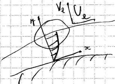
$$V_e \frac{\partial V_e}{\partial x} + V_e \frac{\partial V_e}{\partial y} = -\frac{1}{\rho} \frac{dp_e}{dx}$$
