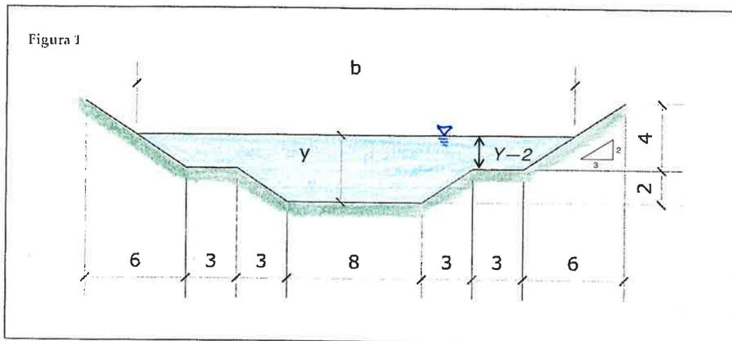
$$E = Y + \frac{Q^2}{2g\Omega^2} \quad (1) \quad Q_0 = \text{cost} = 150 \text{ m}^3 / \text{s}$$
