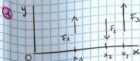
$$\begin{aligned} F_1 &= 500 \text{ N} & x_1 &= 5 \text{ m} \\ F_2 &= 800 \text{ N} & x_2 &= 7 \text{ m} \\ F_3 &= 1000 \text{ N} & x_3 &= 8 \text{ m} \end{aligned}$$
