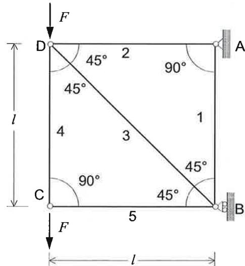
$$[N_1 = 2F = 40 \text{ kN}, N_2 = 2F = 40 \text{ kN}, N_3 = -2\sqrt{2}F = -56.6 \text{ kN}, N_4 = F = 20 \text{ kN}, N_5 = 0;$$
