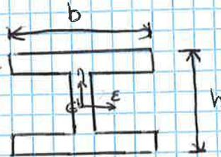
$$\begin{aligned} h &= 120 \text{ mm} \\ b &= 64 \text{ mm} \\ A &= 1,32 \cdot 10^3 \text{ mm}^2 \\ J_{yy} &= 3,18 \cdot 10^6 \text{ mm}^4 \\ J_{xx} &= 2,77 \cdot 10^5 \text{ mm}^4 \end{aligned}$$
