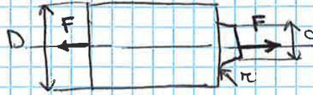
$$\left. \begin{aligned} \frac{r}{d} &= \frac{4}{40} = 0,1 \\ \frac{D}{d} &= \frac{60}{40} = 1,5 \end{aligned} \right\} k_T = 2$$
