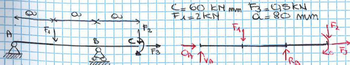
$$\begin{aligned} C &= 60 \text{ kN} \cdot \text{mm} & F_3 &= 0,5 \text{ kN} \\ F_1 &= 2 \text{ kN} & a &= 80 \text{ mm} \end{aligned}$$
