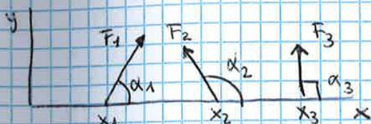
$$\begin{aligned} F_1 &= 100 \text{ N} & x_1 &= 2 \text{ m} \\ F_2 &= 200 \text{ N} & x_2 &= 3 \text{ m} \\ F_3 &= 50 \text{ N} & x_3 &= 4 \text{ m} \\ \alpha_1 &= 60^\circ \\ \alpha_2 &= 135^\circ \end{aligned}$$
