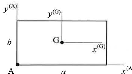
$$[\alpha(p_1^{(G)} \wedge x^{(G)}) = 90^\circ, J_1^{(G)} = 0.667 \cdot 10^4 \text{ mm}^4, J_2^{(G)} = 0.167 \cdot 10^4 \text{ mm}^4, \\ \alpha(p_1^{(A)} \wedge x^{(A)}) = 67.5^\circ, J_1^{(A)} = 3.081 \cdot 10^4 \text{ mm}^4, J_2^{(A)} = 0.253 \cdot 10^4 \text{ mm}^4]$$
