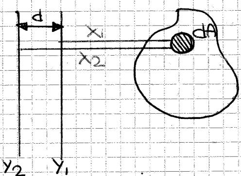
$$\begin{aligned} I_{y_2} &= \int_A x_2^2 dA = \int_A (x_1 + d)^2 dA \\ &= \int_A x_1^2 dA + \int_A d^2 dA + \int_A 2dx_1 dA \\ &= I_{y_1} + d^2 A + 2dS_x \rightarrow \text{MOMENTO STATICO} \end{aligned}$$
