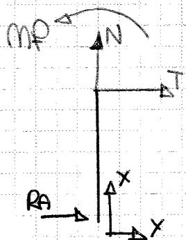
$$\begin{aligned} M_{F_x=0} &= 0 \\ M_F &= -RAx \\ M_F &= \frac{2}{3}e = \frac{qs^2}{2} \cdot \frac{2}{3} = \frac{qs^2}{3} = 2000 \end{aligned}$$
