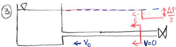
IL FLUIDO SI MUOVE CON VELOCITÀ  $V_0$  MENTRE LA SARACINESCA IMPONE  $V=0$  QUINDI NASCE UNA NUOVA ONDA SIMILE ALLA PRIMA MA QUESTA VOLTA LA LINEA PIEZOMETRICA SI ABBASSA.
