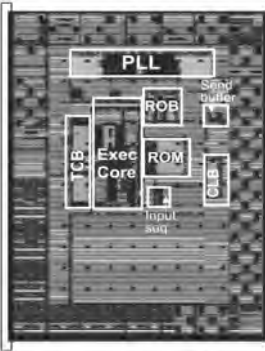
2.23 mm x 3.54 mm, 260K transistors
