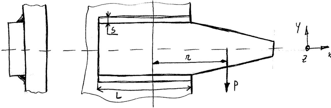
ACCIAIO S275  $r = 500 \text{ mm}$   $h = 180 \text{ mm}$   $L = 240 \text{ mm}$   $s = 18 \text{ mm}$
