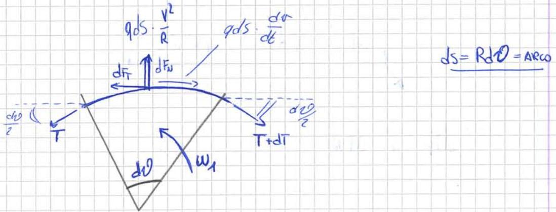
$$\rightarrow) T \cdot \cos \frac{d\theta}{2} + dF_n = (T+dT) \cdot \cos \frac{d\theta}{2} + q ds \frac{dv}{dt} \quad \text{trascurabile}$$
