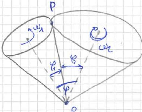
$$z = \frac{\omega_2}{\omega_1} = \frac{v_1}{v_2} = \frac{\sin \varphi_1}{\sin \varphi_2} = \frac{z_1}{z_2}$$
