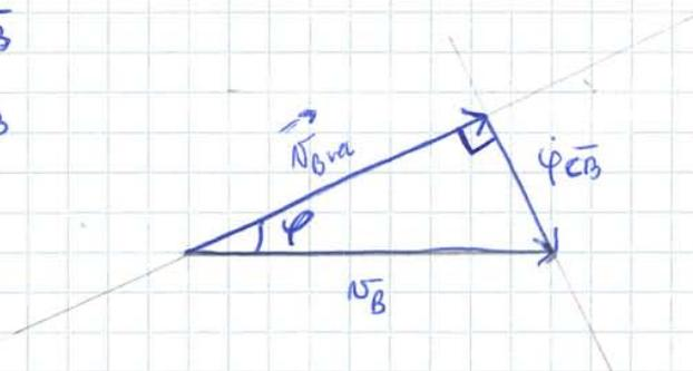
$$v_{B/C} = v_B \cos \alpha = 1,1538 \frac{\text{m}}{\text{s}}$$
