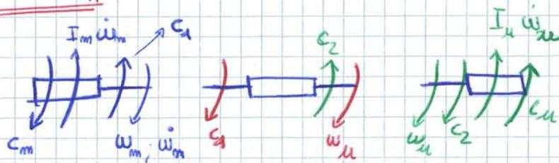
$$\begin{cases} c_m = I_m \dot{\omega}_m + c_1 \\ c_1 \omega_m = c_2 \omega_u \\ c_2 = I_u \dot{\omega}_u + c_u \end{cases}$$
