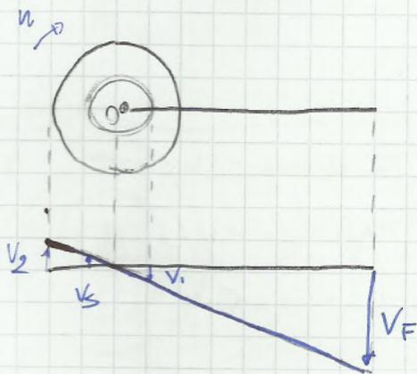
$$v_1 = \omega \frac{d}{2} = 0.62 \text{ m/s}$$
