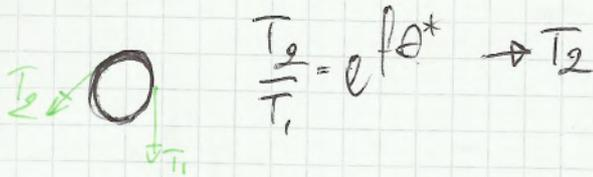
$$\frac{T_2}{T_1} = e^{f\theta^*} \rightarrow T_2$$
