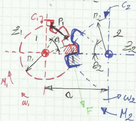
$i = \frac{\omega_1}{\omega_2} = \left(\frac{r_2}{r_1}\right) = \frac{z_2}{z_1}$
