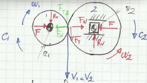
$V_1 = \omega_1 r_1$
