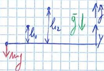
$$\begin{aligned} \bar{x} &= y \cdot \hat{j} & \bar{F}_p &= -m \cdot g \cdot \hat{j} \\ \int_{h_1}^{h_2} \bar{F}_p \cdot d\bar{x} &= \int_{h_1}^{h_2} (-mg \hat{j}) dy = \int_{h_1}^0 (-mg \hat{j}) dy + \int_0^{h_2} (-mg \hat{j}) dy = \\ &= \int_{h_1}^0 (-mg \hat{j}) dy - \int_{h_2}^0 (-mg \hat{j}) dy = V_1 - V_2 = -\Delta V \end{aligned}$$
