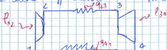
COMPRESSORE - SCAMBIATORE DI CALORE - TURBINA
