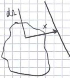
$$M_s = \int_{\Omega} x d\Omega = x_G \Omega$$
