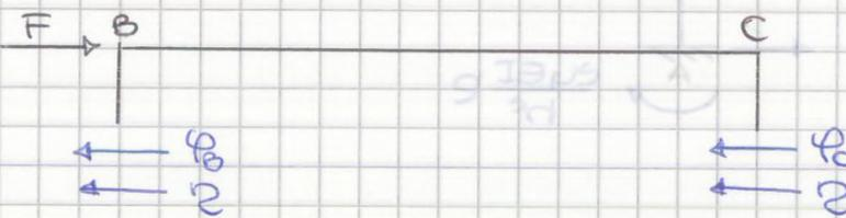
$$\begin{cases} \text{1)} & \frac{16EI}{5} \theta_B + \frac{4EI}{5} \theta_C + \frac{4EI}{5} \theta_B + \frac{2EI}{5} \theta_C + \frac{F}{5} = 0 \\ \text{2)} & \frac{4EI}{5} \theta_C + \frac{6EI}{5} \theta_C + \frac{2EI}{5} \theta_B + \frac{4EI}{5} \theta_C - \frac{F}{5} = 0 \\ \text{3)} & \frac{4EI}{5} \theta_B + \frac{4EI}{h^3} \theta + \frac{6EI}{5} \theta_C + \frac{12EI}{5^3} \theta - F = 0 \end{cases}$$
