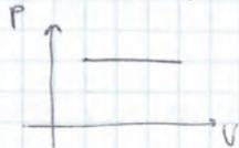
$$\delta Q = ncpdT \quad \text{se rev } \delta W = pdV$$
