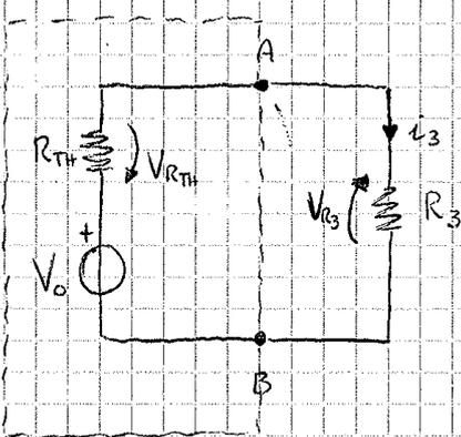
$$\left. \begin{aligned} V_{R_3} + V_{R_{TH}} - V_0 &= 0 \\ V_{R_3} &= R_3 i_3 \\ V_{R_{TH}} &= R_{TH} \cdot i_3 \end{aligned} \right\} i_3 = \frac{V_0}{R_3 + R_{TH}}$$
