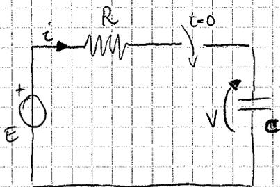
$$E = 10 \text{ V} \quad C = 100 \text{ } \mu\text{F}$$
