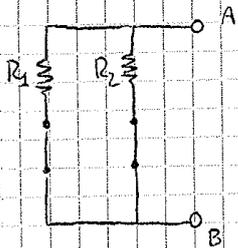
$$R_{eq} = R_{NT} = \frac{R_1 R_2}{R_1 + R_2}$$
