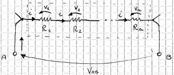
$$\left. \begin{aligned} V_1 &= R_1 i \\ V_2 &= R_2 i \\ V_m &= R_m i \end{aligned} \right\} \text{eq. costitutive}$$
