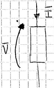
$$\frac{\bar{V}}{\bar{I}} = \bar{Z} \quad \text{IMPEDENZA}$$
