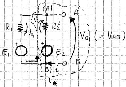
$$\left. \begin{aligned} V_{R_1} &= R_1 i \\ V_{R_2} &= R_2 i \\ E_2 + V_{R_2} + V_{R_1} - E_1 &= 0 \end{aligned} \right\} i = \frac{E_1 - E_2}{R_1 + R_2}$$
