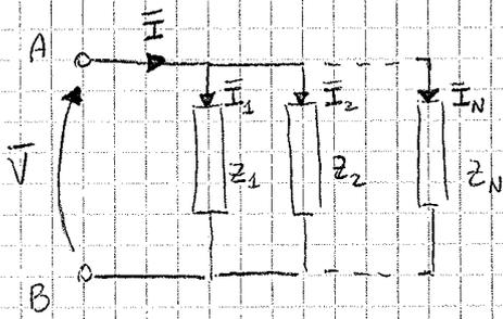
$$\bar{I} = \bar{I}_1 + \bar{I}_2 + \dots + \bar{I}_N$$
