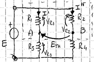
•  $E_{TH} = V_{R2} - V_{R1}$
