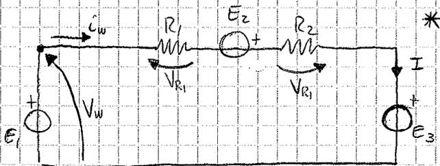
$$\Rightarrow I = i_w \quad \bullet \quad I = \frac{P_W}{V_w} = \frac{120}{30} = 4 \text{ [A]}$$
