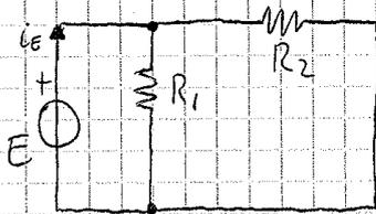
$$R_1 \parallel R_2 \rightarrow R_{eq} = \frac{R_1 R_2}{R_1 + R_2} = 5 \ \Omega$$
