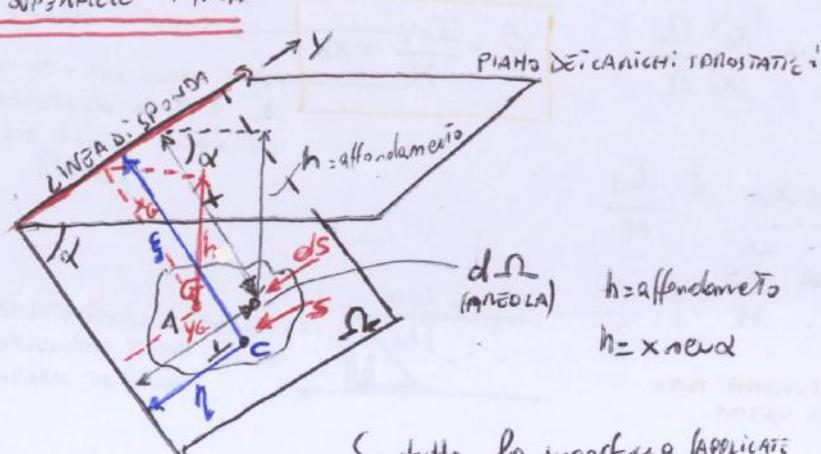
$$S = \int_{\Omega} \vec{P} d\Omega = \int_{\Omega} \vec{\gamma} h d\Omega = \int_{\Omega} \vec{\gamma} x \sin \alpha d\Omega =$$
