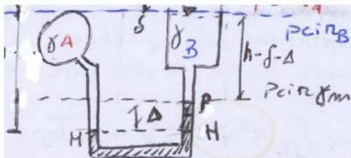
$$P_H = \gamma \cdot h = P_N = P_P + \Delta \gamma_m = \gamma (h - f - d) + \Delta \gamma_m$$
