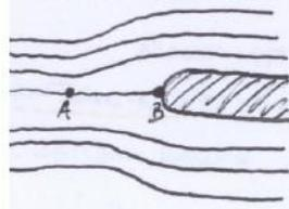
$$\text{BERNOULLI MHD AB} \quad z_A + \frac{p_A}{\gamma} + \frac{u_A^2}{2g} = z_B + \frac{p_B}{\gamma} + \frac{u_B^2}{2g} \quad z_A = z_B + h_A \quad \frac{h_A}{\gamma} = p_A - p_B \quad \text{in A} \\ \frac{h_B}{\gamma} = p_B - p_B \quad \text{in B}$$
