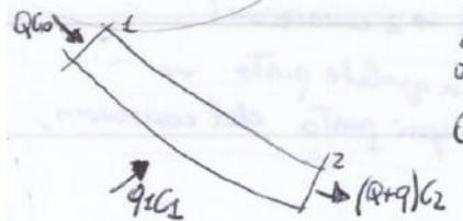
$$Q C_0 + q C_1 = (Q+q) C_2 \rightarrow Q = \frac{C_2 - C_1}{C_2 - C_0} q$$
