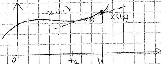
$$\left| \frac{x(t_2) - x(t_1)}{t_2 - t_1} \right| = |\operatorname{tg} \theta|$$
