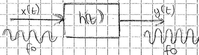
$$\begin{aligned} x(t) &= A_x e^{j(2\pi f_0 t + \varphi_x)} \\ &= A_x e^{j\varphi_x} e^{+j2\pi f_0 t} \end{aligned}$$
