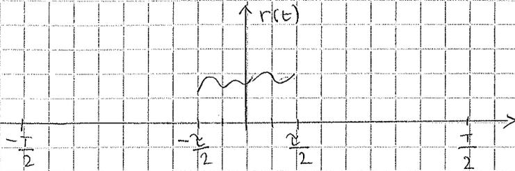
$$\begin{aligned} \mu_n &= \frac{1}{T} \int_{-T/2}^{T/2} x(t) e^{-i2\pi n t} dt = \frac{1}{T} \int_{t_0 - T/2}^{t_0 + T/2} x(t) e^{-i2\pi n t} dt \\ &= \frac{1}{T} \int_{t_0 - T/2}^{t_0 + T/2} r(t - t_0) e^{-i2\pi n t} dt \end{aligned}$$
