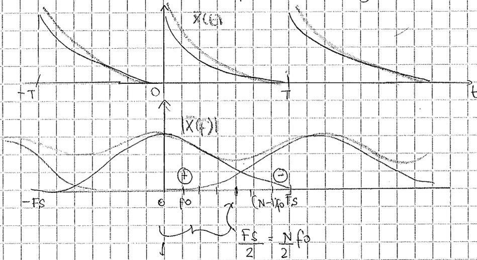
freq. non negative:  $\bar{x}(0), \bar{x}(f_0), \dots, \bar{x}(N/2 f_0)$
