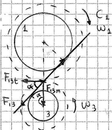
$$\eta = 1 = \frac{C_3 \omega_3}{C_1 \omega_1} = \frac{C_3 \omega_3}{P} \Rightarrow C_3 = 97,5 \text{ Nm}$$
