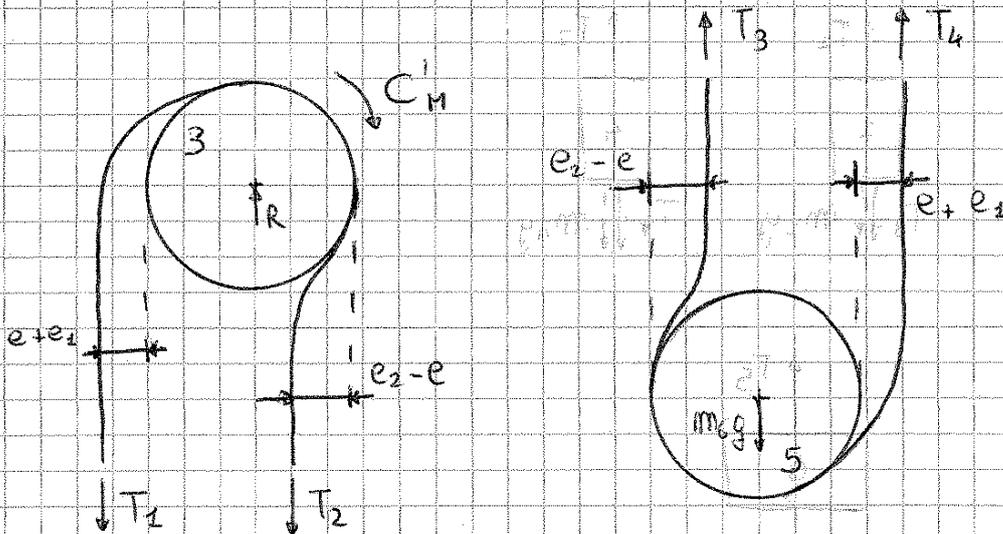
$$\begin{cases} C_M = T_1 \cdot (R_3 + e + e_1) - T_2 \cdot (R_3 - e_2 + e) \\ T_1 = T_3 + m_1 g \\ T_2 = T_4 + m_4 g \\ T_3 + T_4 = m_0 g \\ T_3 (R_5 - e_2 + e) = T_4 (R_5 + e + e_1) \end{cases}$$
