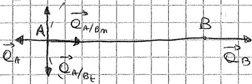
$$\vec{Q}_A = \vec{Q}_B + \vec{Q}_{A/Bm} + \vec{Q}_{A/Bt}$$
