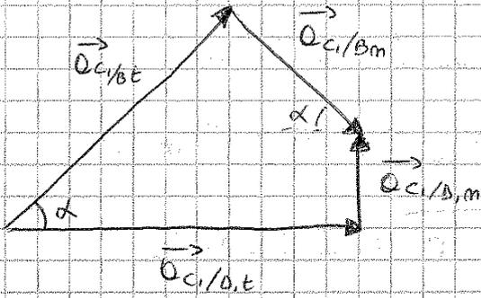
$$Q_{C1/D,t} = Q_{C1/B,m} \cos \alpha + Q_{C1/D,t} \cos \alpha = \cos \alpha (Q_{C1/B,m} + Q_{C1/D,t})$$
