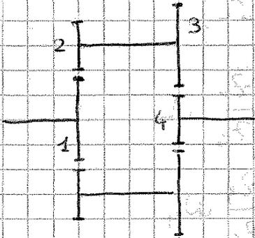
$$\frac{\omega_1 - \omega_u}{\omega_u - \omega_u} = -\frac{z_2}{z_1} \cdot \left( -\frac{z_4}{z_3} \right)$$
