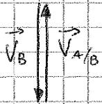
$$V_B = V_{A/B} = 10 \text{ m/s} \Rightarrow V_A = 0$$
