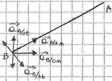
$$\vec{v}_B = \vec{v}_A + \vec{v}_{B/At} + \vec{v}_{B/a/m}$$
