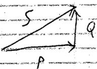
$$|S| = \sqrt{P^2 + Q^2} = \frac{1}{2} |V| |I| = A \quad \text{Pot. apparente}$$
