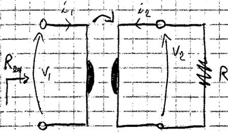
$$R_{eq} = \frac{V_1}{i_1} = \frac{1}{g_m} \frac{1}{R}$$
