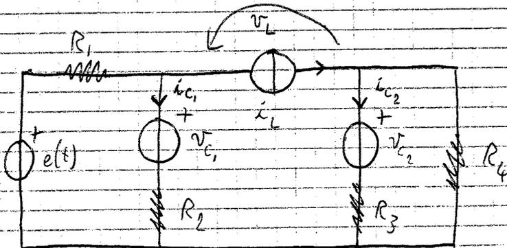
$$i_{c1} = \frac{-v_{c1}}{R_1 + R_2} - i_L \frac{R_1}{R_1 + R_2} + \frac{e(t)}{R_1 + R_2} \quad v_L = \frac{v_{c1} R_1}{R_1 + R_2} - \frac{v_{c2} R_4}{R_3 + R_4} - L \left( \frac{R_1 // R_2 + R_3 // R_4}{R_1 + R_2} \right) + e(t) \frac{R_2}{R_1 + R_2}$$
