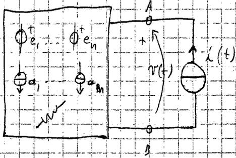
$$v(t) = \alpha_1 e_1(t) + \alpha_2 e_2(t) + \dots + \alpha_n e_n(t) + \beta_1 a_1(t) + \dots + \beta_m a_m(t) + \gamma i(t)$$
