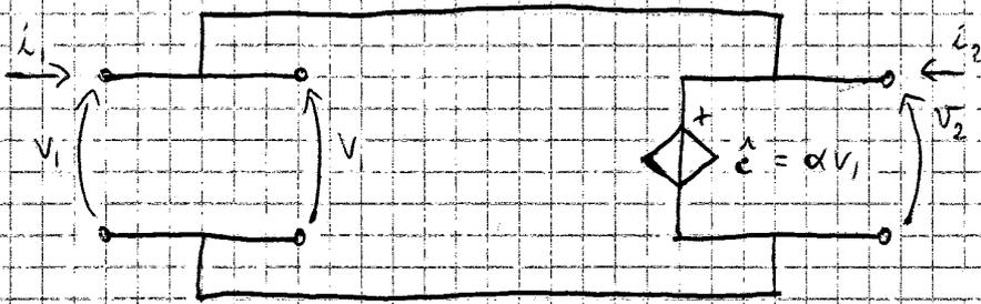
$$\begin{cases} i_1 = 0 \\ v_2 = \hat{e} = \alpha v_1 \end{cases} \quad \begin{pmatrix} i_1 \\ v_2 \end{pmatrix} = \begin{pmatrix} 0 & 0 \\ \alpha & 0 \end{pmatrix} \begin{pmatrix} v_1 \\ i_2 \end{pmatrix}$$
