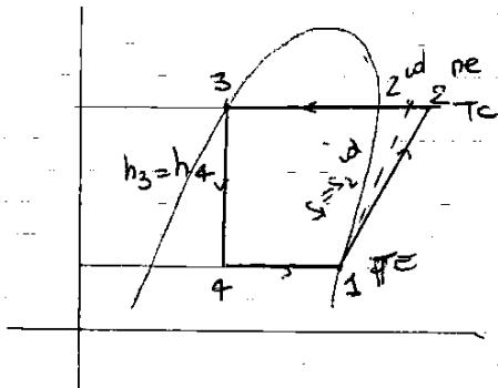
$$\text{COP} = \frac{h_1 - h_4}{h_2^{\text{id}} - h_1}$$
