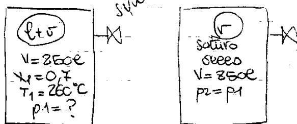
$$\textcircled{1} \quad T = 260^\circ\text{C} \quad p_1 = 46,943 \text{ Bar} = p_2$$
