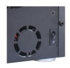
4. With the power cord connected to the power source, turn on the RocketStor 6628T using the power switch on the rear panel (switch to the "I" position to power on the RocketStor 6628T).
