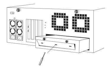
2. Unscrew the four screws on L-type bracket on plate drawer, place the Mac mini Server into drawer, and restore the L-type bracket to fasten Mac mini Server with drawer.
