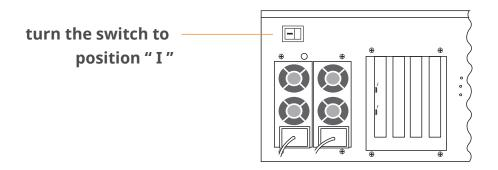
2. The HighPoint NA381TB3 is designed to be powered on/off simultaneously with Thunderbolt Mac when storage is connected to Mac by Thunderbolt cable. Therefore, power on Mac first, and then NA381TB3 will be powered on automatically. (HighPoint NA381TB3 also supports hot-plug and hot-unplug for powering on and off)
