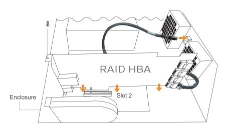
5. Connect the cable between the topmost mini-SAS connector on backplane and the mini-SAS connector Channel 1~4 on RAID card, and then connect the rest cables subsequently to the bottommost one on backplane and Channel 21~24 on RAID card.
