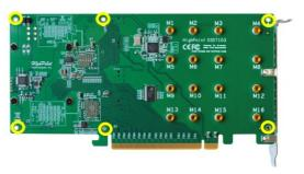
After removing the screws, carefully remove the front panel from the SSD7103.
