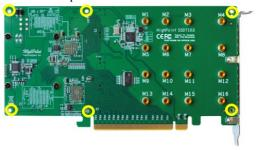
**Note:** Make sure the aluminum cover is properly aligned with the controller board (PCB), and that it makes full contact with the thermal pad, before refastening it to the SSD7103. If the cover is improperly
