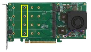
Step 4. The SSDs should be installed from top to bottom. Remove the top screw.
