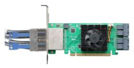
2. The other end of the SFF-8644 to SFF-8644 connects to the RS6444 SFF-8644 connector as illustrated below (a to a, and b to b), RS6444 connects to U.2 NVMe, and connect to AC power;
