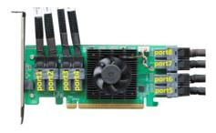
*Note:* Please make sure the cables are securely connected to the R1180's device ports and the NVMe SSDs or backplane. Loose connections can lead to a variety of problems including instability, slower than expected performance and dropped disks.
