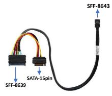
Step 4: Shown above is an SFF-8643 to U.2 SFF-8639 cable with a 15pin SATA power connector. Connect the R1120 to the NVMe SSD's using the appropriate SFF-8643 cables. The SFF-8639 port should be connected to the NVMe SSD's U.2 port. The 15 pin SATA power connector should be connected the system's power supply.
