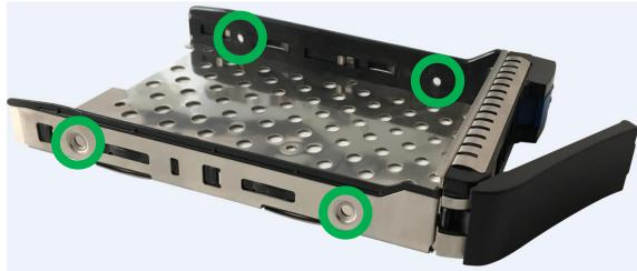
2. If using 2.5" SSDs, please use the 2.5" mounting screws to connect the SSDs to the tray in the locations shown below
