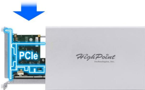
Step 3: Close the RocketStor 6661A chassis and connect the Power Adapter to the RocketStor 6661A.
