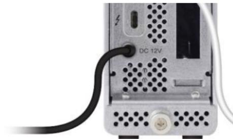
Step 2: Connect the RocketStor 6661A-4USB to the host system using a Thunderbolt™ cable.
