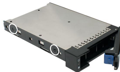
Figure 2. HDD mount points (side)
