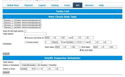
The **Health Inspector Scheduler (HIS)** enables you to schedule disk/array checkups to ensure disks/array are functioning optimally.
