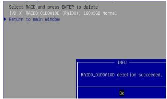
Warning: All data stored on the array will be lost – do not delete if the array contains critical data.
