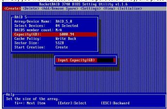
Note: Multiple arrays can be created using the same set of hard disk drives. The Capacity option allows you to set aside disk space that be used to create another array, set as a spare disk, or partitioned to act as a single disk (by the operating system).
