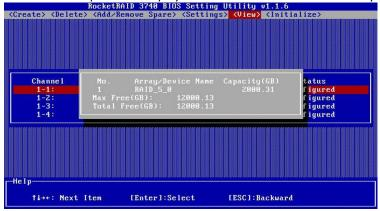
**RAID Array** – This option will display information about each RAID array hosted by the HBA. Highlight the target device and press the Enter key to view details about the configuration.
