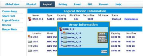
An array with the Disabled status means that the RAID level does not have enough disks to function.
