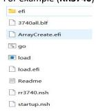
**Note:** If the above content is not present in the root directory, the UEFI boot device will not be properly recognized
