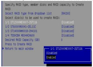
Note: Disks don't need to be initialized before they can be used to create arrays.
