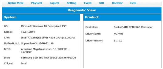
It also provides one-click collection of controller information, and the collected content information is packaged into a compressed package and saved in the C drive. Log Location will show you where to save the log in detail.
