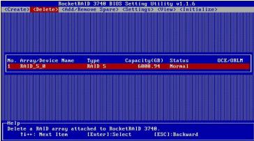
The utility will display a warning message. Press Y (yes) to delete the array, or select N (no) to cancel. **Warning**: All data stored on the array will be lost – do not delete if the array contains critical data.
