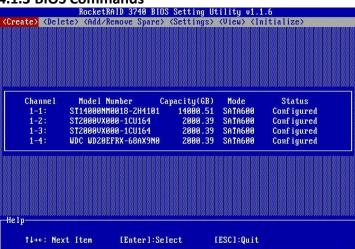
**Create**: This command is used to create the RAID array.
