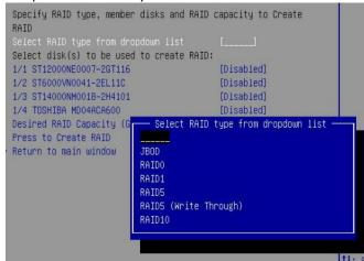
Supported RAID Type: JBOD/ RAID0/RAID1/RAID5/RAID5(Write Through)/ RAID10
