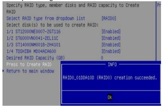
Note: Multiple arrays can be created using the same set of hard disk drives. The Capacity option allows you to set aside disk space that be used to create another array, set as a spare disk, or partitioned to act as a single disk.
