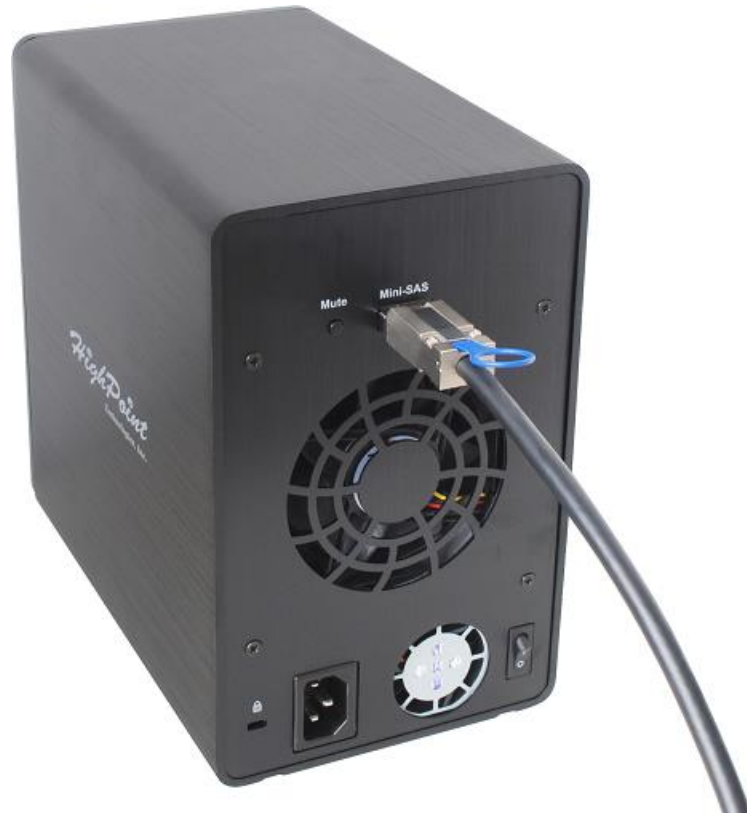
Mini-SAS connection on RocketStor 6414S enclosure back panel
