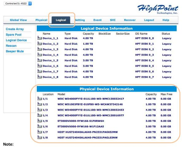
Single or new (unused) drives will be labeled as Legacy disks. Legacy disks can be used to create a new RAID array.
