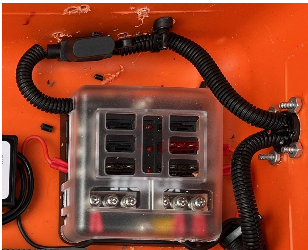
Figure 22 – Fuse block mounted near power connector
