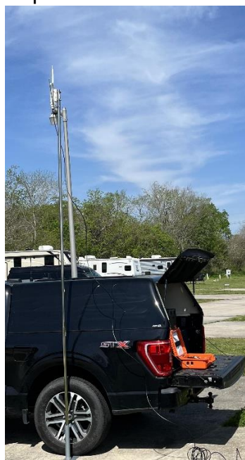
Figure 37 – Antenna mast with Wi-Fi device assembled and mounted.
