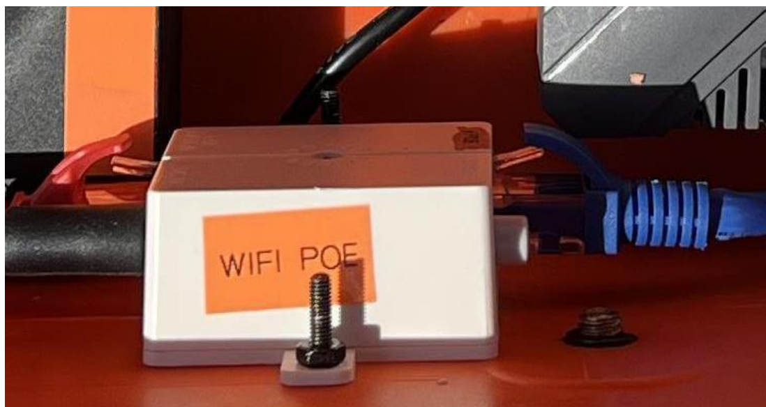
Figure 32 – Installation of the POE adapter in the Hard Case
