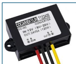
Figure 29 – 12 to 24-volt power supply for POE adapter
