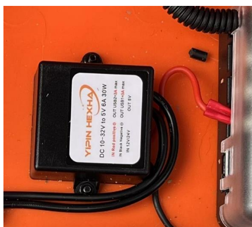
Figure 25 – 12-volt to 5-volt USB-C power supply
