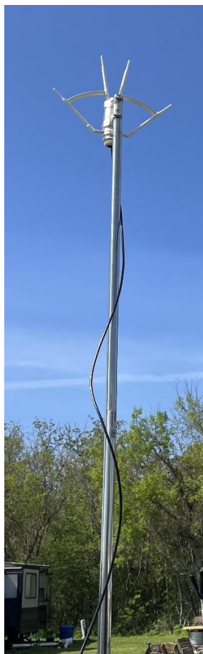
Figure 34 – Assembled Wi-Fi extender on antenna mast with tire base
