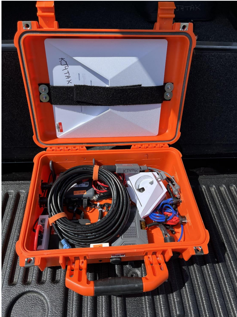
Figure 8 Inside the hard case with all of the components required to function. Notice the lid contains the Starlink Mini
