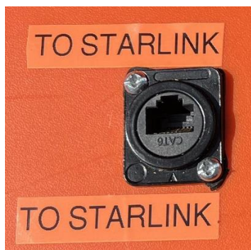
Figure 17 – Starlink Mini Power and Network Connection
