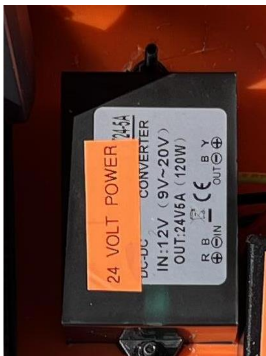
Figure 25a – DC to DC converter 24-Volts output.
