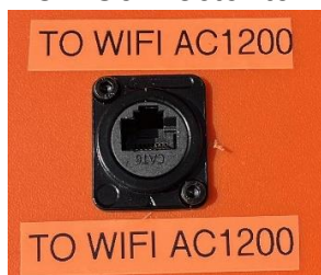
Figure 17a – POE Connection for Wi-Fi Extender Only
