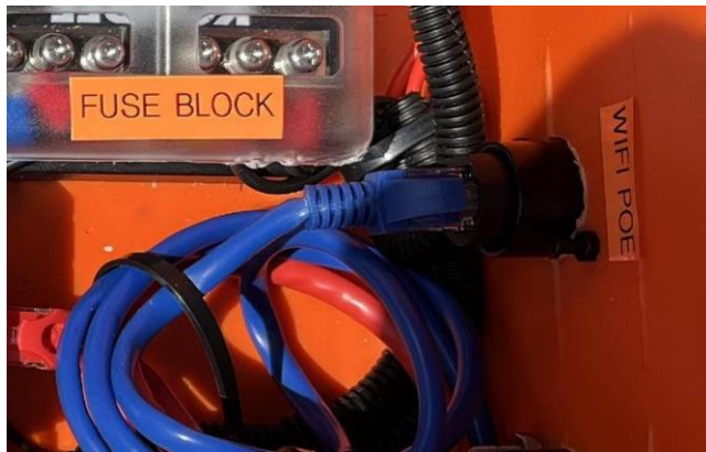
Figure 33 – External network port for POE power
