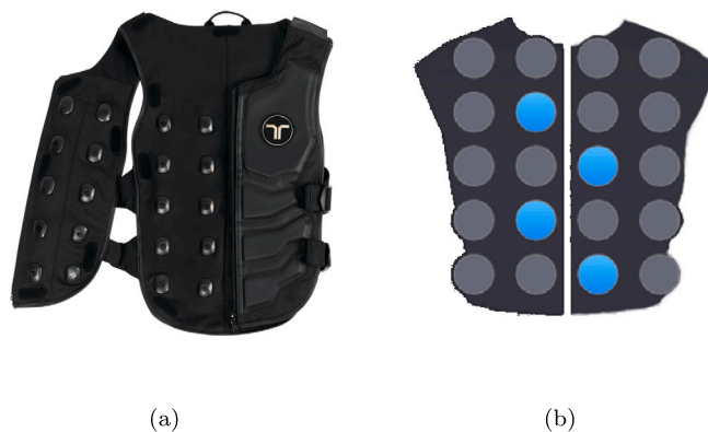
Fig. 4. Wearable and portable haptic suit with a double vibration motors matrix: (a) suit, (b) front view of matrix with motors.
