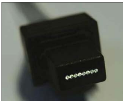
Fig. 7 – Ribbon POF com 8 x 500 \mu\text{m} POF
