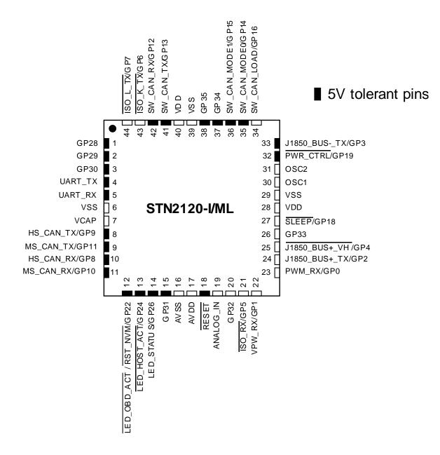
Note 1. The metal plane at the bottom of the device is not connected to any pins and is recommended to be connected to Vss externally.
