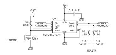
The only additional components are the decoupling capacitor C10, and the EMI filters R21/C11 and R22/C12.
