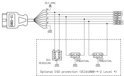
Figure 9 - STN2100 OBD Port Connector and ESD Protection
