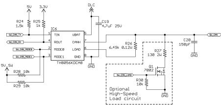
Figure 19 - Single Wire CAN Transceiver
