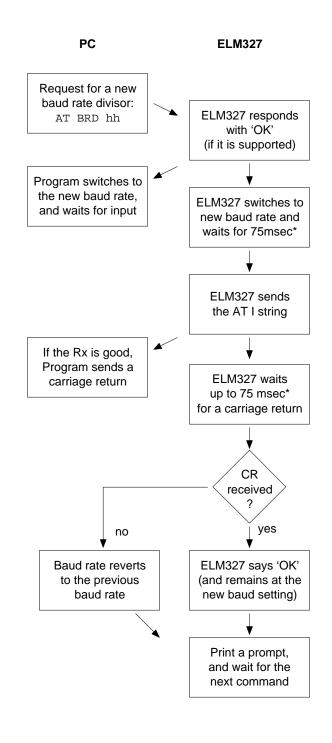
\* Note that the 75msec time is adjustable (with the AT BRT hh command)
