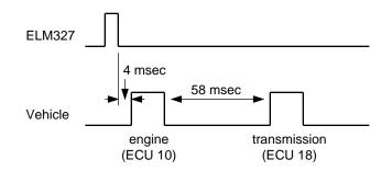
The engine responds very quickly, but the transmission takes considerably longer. The adaptive timing algorithm measures the longer transmission response times and will use them to set the timeout, likely to a value in the range of 90msec. With a timeout of 90 msec, the maximum scan rate may be about 6 readings per second.
