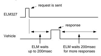
The ELM327 sends a request then waits up to 200msec for a reply. If none were to come, an internal timer would stop the waiting, and the ELM327 would print "NO DATA".
