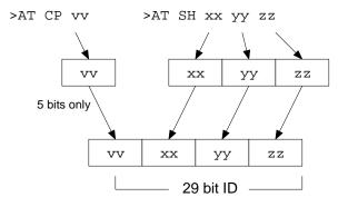
Figure 5. Setting a 29 bit (extended) CAN ID
