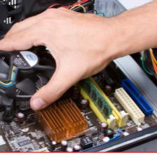
Mount the motherboard on its place (Use the plastic pieces only if necessary).
