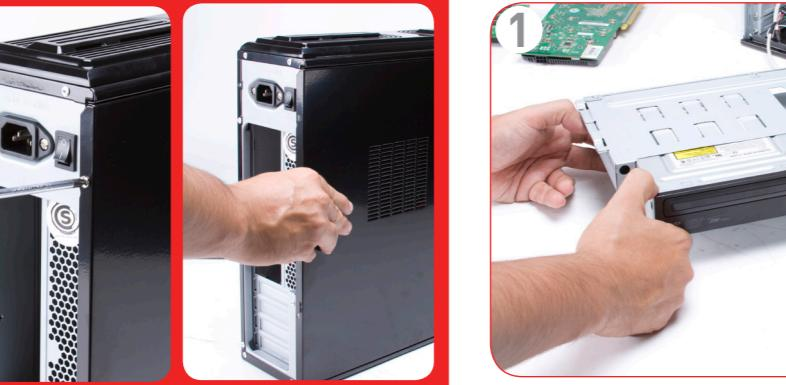
Extract the 4 screws and slide the cover towards the back side of the case. Lift the cover.
