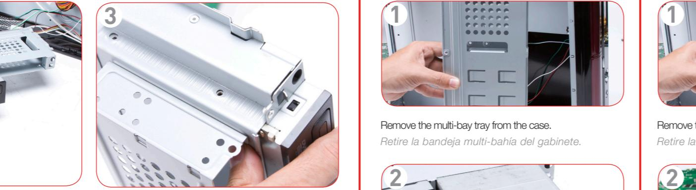
Withdraw the multi-bay tray from the case and insert the optic drive in the corresponding bay.
