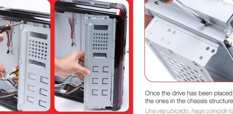
To remove the multi-bay tray, unscrew it from the chassis and lift up.
