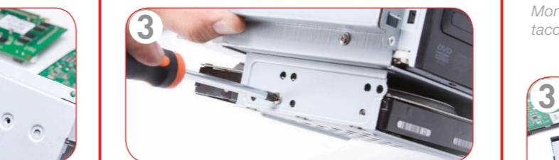
Adjust the screws until the drive is firmly held.
