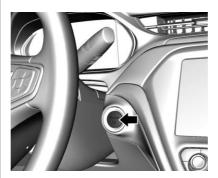
The vehicle has an electronic pushbutton start.
