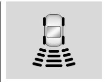
The instrument cluster may have a Park Assist display with bars that show "distance to object" and object location information for RPA. As the object gets closer, more bars light up and the bars change color from yellow to amber to red. When an object is first detected in the rear, one beep will be heard from the rear. When an object is very close, <0.6 m (2 ft) in the vehicle rear, five beeps will sound from the rear depending on object location.
