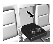
If equipped, lower the armrest to access the rear cupholders. The liner is removable for cleaning.
