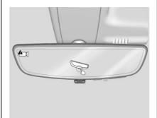
See your dealer for service if a blue screen and are displayed in the mirror, and the display shuts off. Also, push the tab as indicated to return to the automatic dimming mode.
