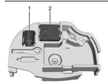
Remove the tire sealant canister (1) and the compressor (2).
