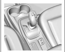
The vehicle uses an electric drive unit. The shift lever always starts from a center position. An amber dot is displayed on the shift pattern. After releasing the shift lever, it will return to the center position.
