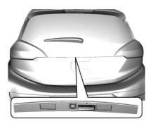
To open the liftgate, press the touch pad and lift up.
