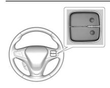
The volume switches are on the right rear side of the steering wheel. Press to increase or decrease the volume.
