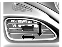
Move the slats to change the direction of the airflow.
