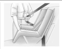
Pull the shoulder belt all the way out of the retractor to set the lock. When the retractor lock is set, the belt can be tightened but not pulled out of the retractor.
