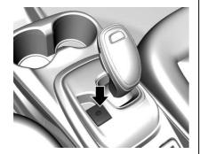
The vehicle has an Electric Parking Brake (EPB). The EPB can always be activated, even if the vehicle is off.
