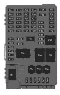
The instrument panel fuse block is on the left side of the instrument panel. To access the fuses, open the fuse panel door by pulling out.
