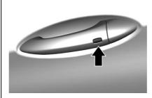
Pressing the lock/unlock button will cause all doors to lock if any of the following occur:
