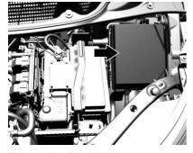
To open the fuse block cover, press the clips at the side and back and pull the cover up.
