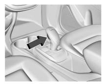
This vehicle is equipped with an electric drive unit. The shift lock release button is designed to prevent inadvertent shifting out of P (Park) unless the ignition is on, the brake pedal is applied, and the shift lock release button is pressed.
