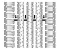
Treadwear indicators are one way to tell when it is time for new tires. Treadwear indicators appear when the tires have only 1.6 mm (1/16 in) or less of tread remaining. See *Tire Inspection* ⇒ 272 and *Tire Rotation* ⇒ 273.
