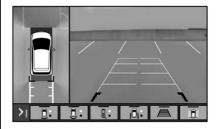
Touch the camera view buttons along the bottom of the infotainment display.
