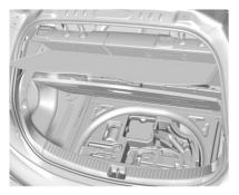
Pull up on the load floor cover to access the cargo management system, if equipped. There is a carpeted open storage area. Remove the carpet and the cover to access additional storage.
