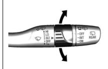
**INT**: If equipped with intermittent wipes, move the windshield wiper lever to INT. Turn the band up for more frequent wipes or down for less frequent wipes.
