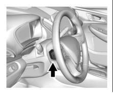
There is a paddle on the left rear side of the steering wheel for regenerative braking. See Regenerative Braking \$\dip\$ 217.
