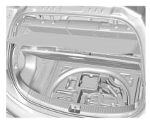
Pull up on the load floor cover to access the cargo management system, if equipped. There may be a carpeted open storage area. Remove the carpet, if equipped, and the cover to access additional storage.
