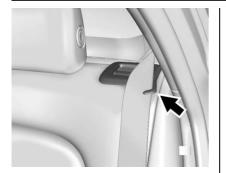
Make sure the seat belt is in the retainer hook.
