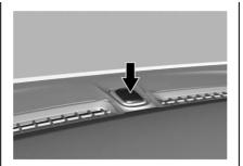
There is a light sensor on top of the instrument panel. Do not cover the sensor, otherwise the headlamps will come on when they are not needed.
