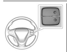
The volume switches are on the right rear side of the steering wheel. Press to increase or decrease the volume.
