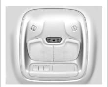
The dome lamp controls are in the overhead console above the front seats.
