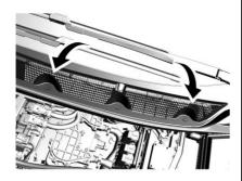
The air intake at the base of the windshield under the hood must be kept clear to allow the flow of air into the vehicle. Clear away any ice, snow, or leaves.
