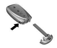
Press the key release button to extend the key. The key can be used for all locks.
