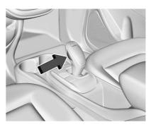
This vehicle is equipped with an electric drive unit. The shift lock release button is designed to prevent inadvertent shifting out of P (Park) unless the ignition is on, the brake pedal is applied, and the shift lock release button is pressed.
