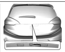
To open the liftgate, press the touch pad on the underside of the liftgate and lift up.
