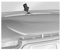
The vehicle has a Charging Status Indicator (CSI) at the center of the instrument panel near the windshield. When the vehicle is plugged in and vehicle power is off, the CSI indicates the following:
