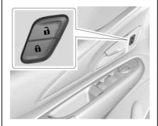
To lock or unlock the liftgate from the inside, press  $\widehat{\ensuremath{\mathbf{a}}}$  or  $\widehat{\ensuremath{\mathbf{a}}}$ .
