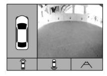
If equipped, a view of the area in front of the vehicle appears in the infotainment display. The front view shows after shifting from R (Reverse) to D (Drive) and when the vehicle is moving forward slower than 8 km/h (5 mph).
