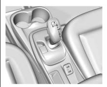
The vehicle uses an electric drive unit. The shift lever always starts from a center position. An amber dot is displayed on the shift pattern. After releasing the shift lever, it will return to the center position.
