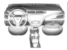
The driver knee airbag is below the steering column. The front outboard passenger knee airbag is below the glove box.
