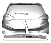
To open the liftgate, press the touch pad and lift up.
