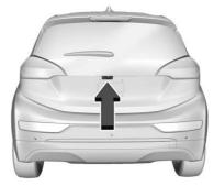
The camera that provides the Rear Camera Mirror (RCM) image is above the license plate, next to the Rear Vision Camera (RVC).
