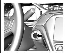
The vehicle has an electronic pushbutton start.
