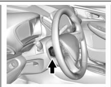
There is a paddle on the left rear side of the steering wheel for regenerative braking. See Regenerative Braking ♀ 217.
