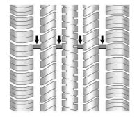
Treadwear indicators are one way to tell when it is time for new tires. Treadwear indicators appear when the tires have only 1.6 mm (1/16 in) or less of tread remaining. See *Tire Inspection*  $\Rightarrow$  291 and *Tire Rotation*  $\Rightarrow$  292.
