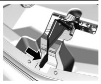
Go to the front of the vehicle and locate the secondary release lever under the front center of the hood. Push the secondary hood release lever to the right to disengage.
