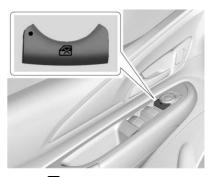
Press on the driver door to activate the window lockout. The indicator light in the switch will illuminate when activated.
