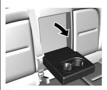
If equipped, lower the armrest to access the rear cupholders. The liner is removable for cleaning.
