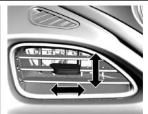
Move the slats to change the direction of the airflow.
