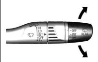
The controls are on the end of the windshield wiper lever.
