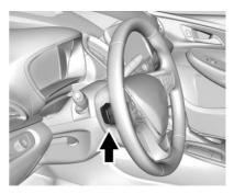
This feature is activated using the steering wheel paddle. Regen on Demand slows the vehicle by recapturing energy.
