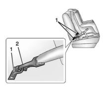
Lower anchors (1) are metal bars built into the vehicle. There are two lower anchors for each LATCH seating position that will accommodate a child restraint with lower attachments (2).
