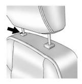
To lower the head restraint, press the button on the top of the seatback and push the head restraint down. Try to move the head restraint after the button is released to make sure it is locked in place.
