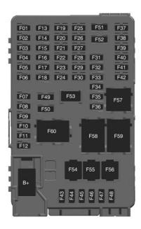
The instrument panel fuse block is on the left side of the instrument panel. To access the fuses, open the fuse panel door by pulling out.
