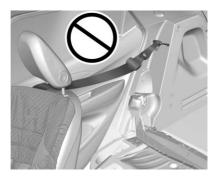
Do not attach the top tether to this location. Use only the approved top tether anchors identified previously in this section.
