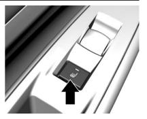
If equipped, the rear heated seat buttons are on the rear doors.
