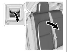
Pull the lever on top of the seatback to unlock the seatback.
