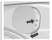
Push the rearward edge of the charge port door and release to open the door.
