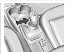
The shift lock release button is designed to prevent inadvertent shifting out of P (Park) unless the vehicle has been started, the brake pedal is applied, and the shift lock release button is pressed.
