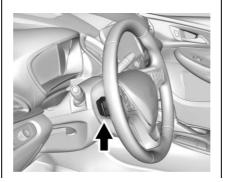
Regen on Demand allows increased deceleration by pressing and holding the steering wheel paddle. It works in D (Drive) and L (Low). The accelerator pedal can be used to manage deceleration while using Regen on Demand.
