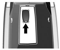
Open the center console and take out the small tray, if equipped. Place the two recognized transmitters in the backup location with the buttons facing down. The DIC displays READY FOR REMOTE # 3, 4, 5, 6, 7, or 8.
