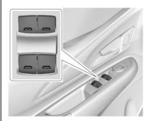
Press the switch to open the window. Pull the front of the switch up to close it.
