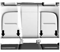
The outboard lower anchors are behind the vertical openings in the rear seat trim.
