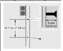
Mark and drill the mounting holes in a wall stud or suitable structure. Stay away from any power source.
