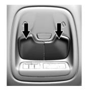
The front reading lamps are in the overhead console.
