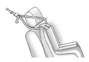
If the position you are using has an adjustable headrest or head restraint and you are using a dual tether, raise the headrest or head restraint and route the tether under the headrest or head restraint and around the headrest or head restraint posts.
